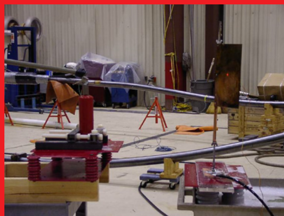
Figure 2. General Setup Illustrating Test Extinguisher and Target
