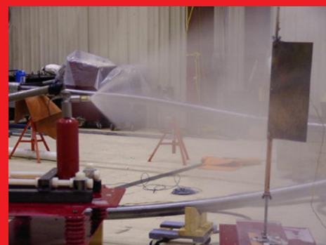
Figure 5. 0.8-L FOG1 Extinguisher UL 711 (Class C) - Test in Progress
