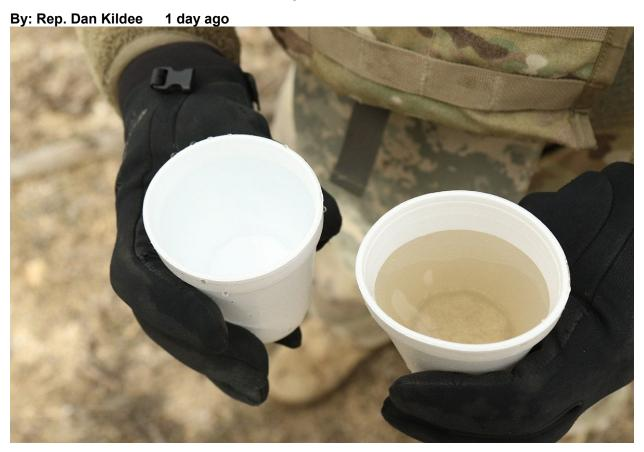
A water purification specialist shows an up-close comparison of water before and after purification at the Tactical Water Purification System site on Jan. 25, 2019, during Pegasus Forge IV on Fort Hood, Texas. (Spc. Calab Franklin/Army)
