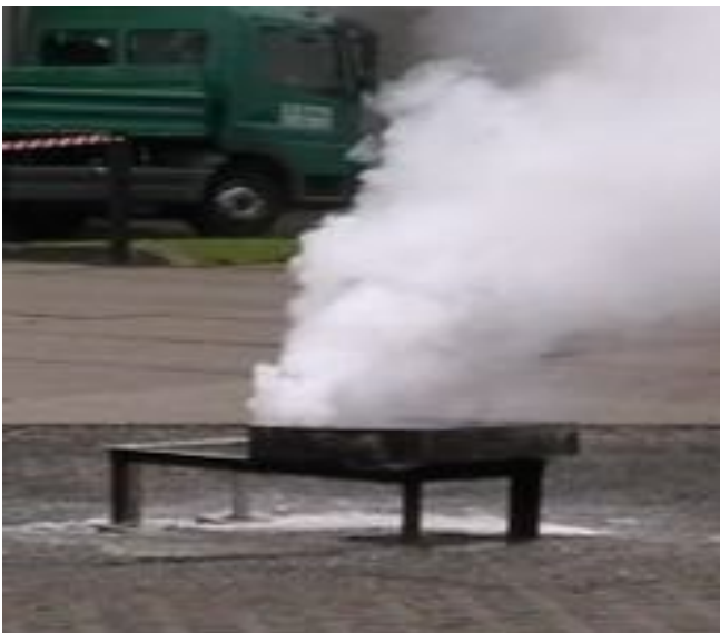
(10:16) First phase ends – fire is out (Surface temp. is high at this stage)
