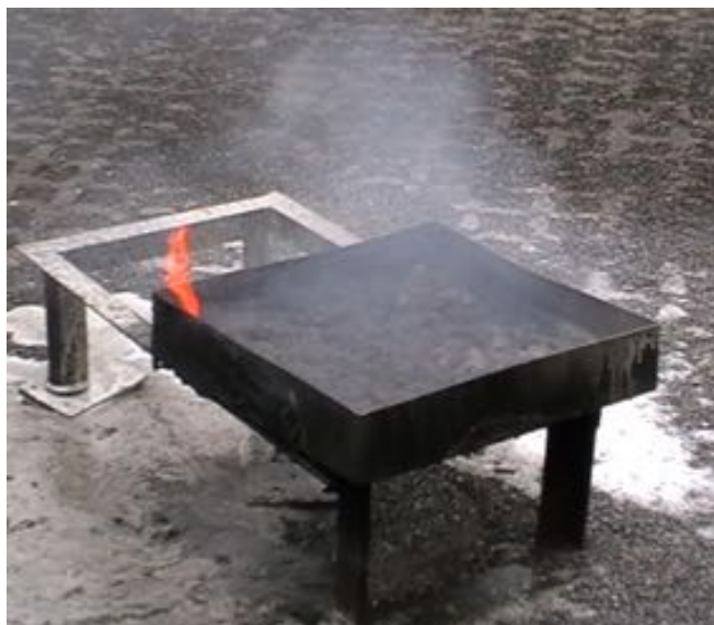
2 nd phase: 11:35 the chemical reaction release volatile gases ignite as the bubbles burst
