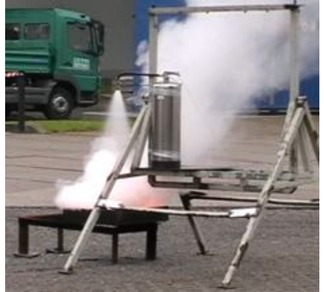
(7:45) 9-ltr extinguisher sprays on & off seq. (25-sec; 6-sec; 27-sec; 22-sec; 16-sec)
