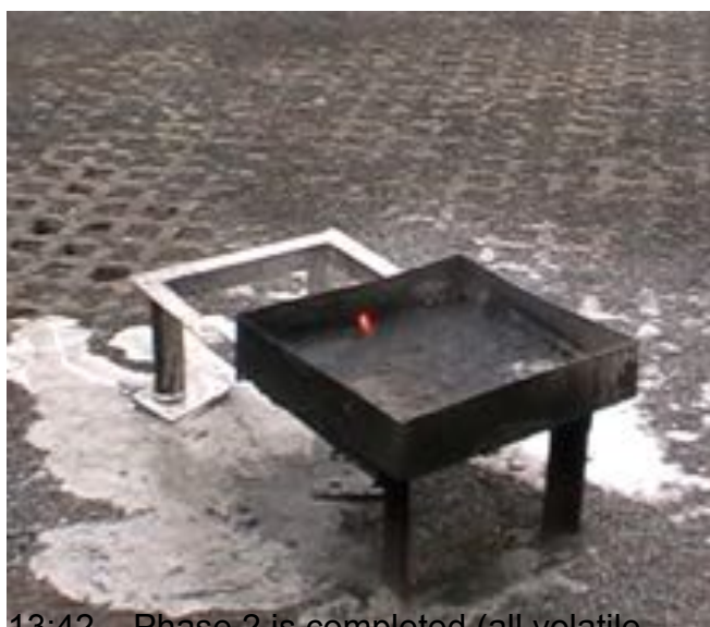
13:42 – Phase 2 is completed (all volatile gases are burned off)
