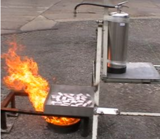
2-Kg of sodium metal – heated to auto ignition (It took approx. 6-min to ignition)
